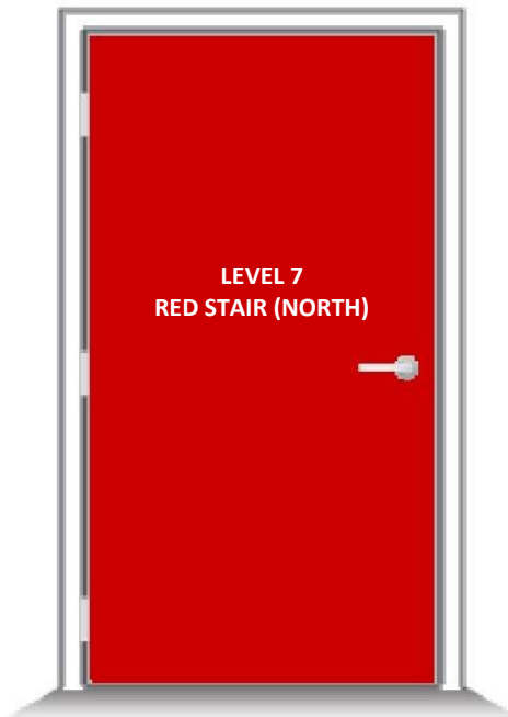
Figure 2: Scissor stair fire door identification - internal (stair side) face of fire stair door.
